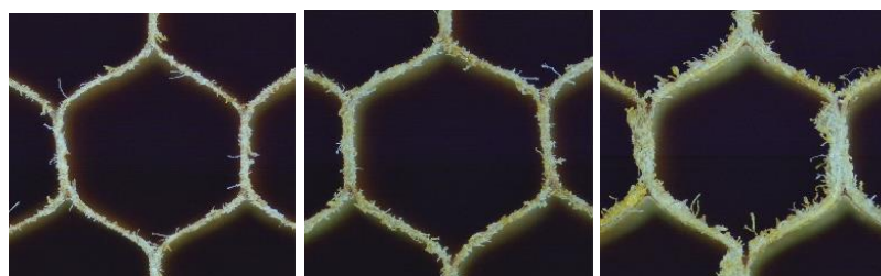
FIGURE 3. Burrs of different severity levels (a) fewer burrs (b) moderate burrs (c) more burrs.
