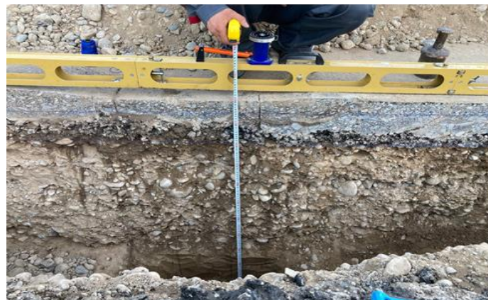
FIGURE 2. Measuring thicknesses of the pavement layers
