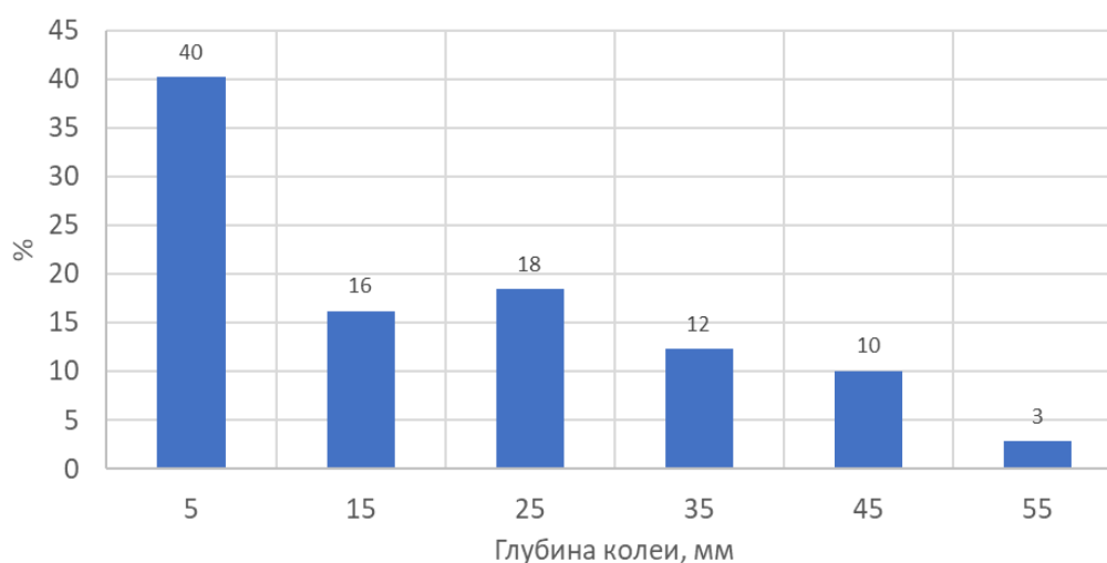
FIGURE 5. Histogram of distribution of rut depth on the asphalt concrete surface on the experimental section
