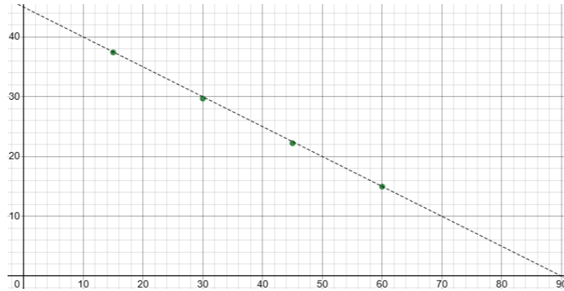
FIGURE 13. Comparison of the internal friction angle vs shear band inclination angle for the analytical (solid line) and numerical (dots) solutions.
