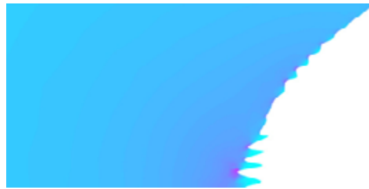
FIGURE 1. Example of false loss of stability of the shape of an initially circular corroding surface.
