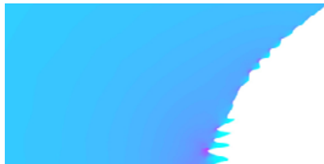
FIGURE 1. Example of false loss of stability of the shape of an initially circular corroding surface.
