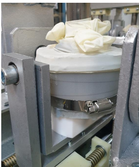
FIGURE 12. Test station bath with the prosthesis being tested inside
