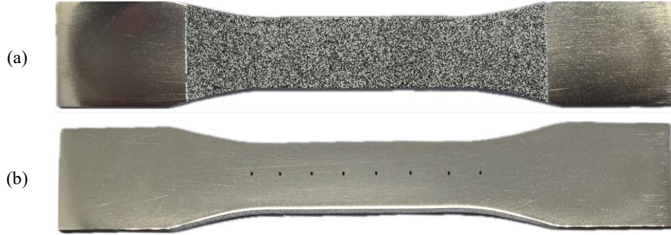
FIGURE 2. Specimen surfaces prepared for DIC analysis (a) and contact profilometry (b)
