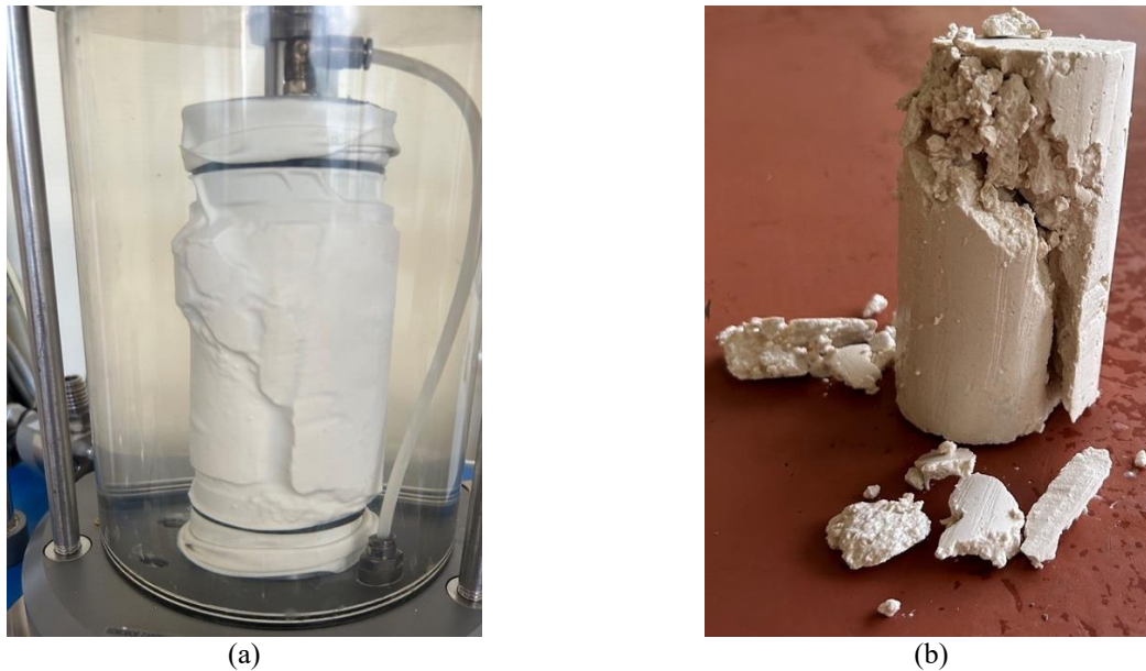
FIGURE 1. Results of experiment No. 4 on selecting a recipe for equivalent material: (a) view of the sample in the triaxial compression device after the end of the experiment, (b) view of the sample after removal from the device.
