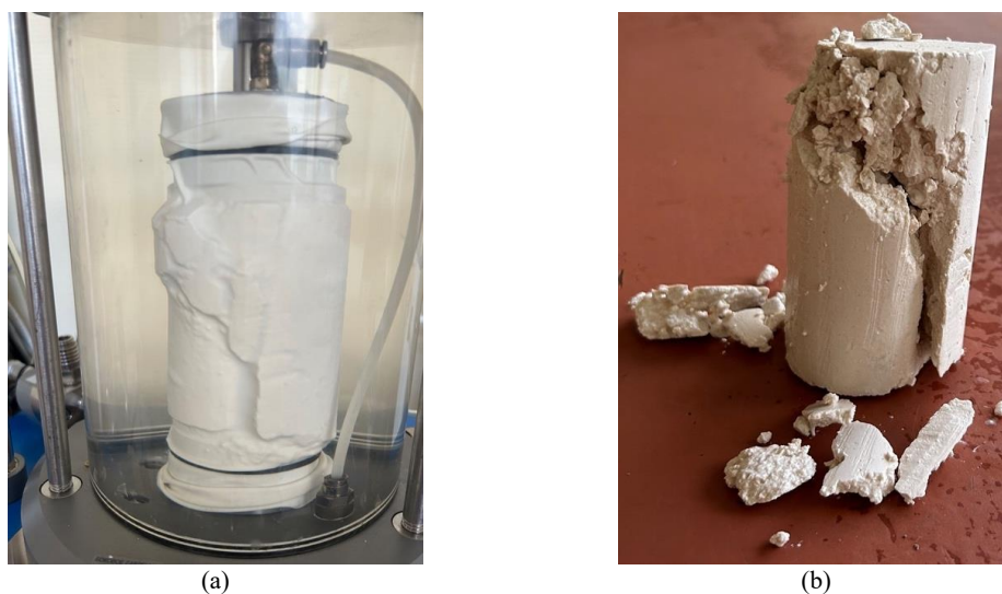
FIGURE 1. Results of experiment No. 4 on selecting a recipe for equivalent material: (a) view of the sample in the triaxial compression device after the end of the experiment, (b) view of the sample after removal from the device.
