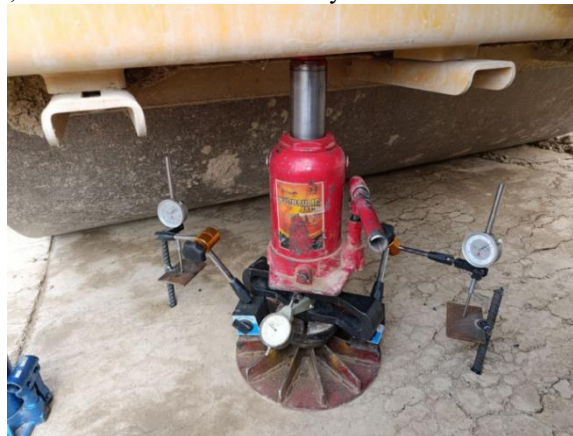
FIGURE 1. Process of stamping test of composite soils.
