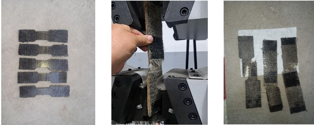
FIGURE 2. The samples of carbon and basalt tapes before and after testing
