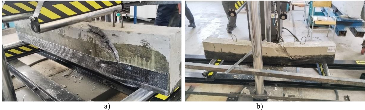
FIGURE 4. Destruction of samples reinforced without clamps: a) carbon tape, b) basalt tape
