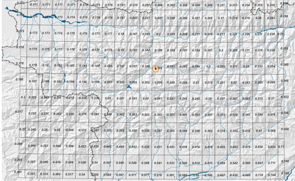
FIGURE 6. Peak ground acceleration (PGA) for 10% probability of exceedance in 50 years (475 years return period) for every cell of the matrix
