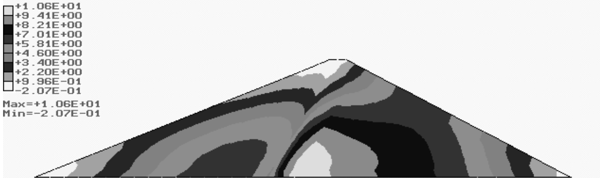
FIGURE 5. Isolines of principal stresses in the first high earth dam according to the first mode of vibrations
