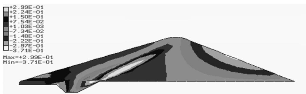
FIGURE 6. Isolines of the principal normal stresses of the earth dam according to the first mode of vibration
