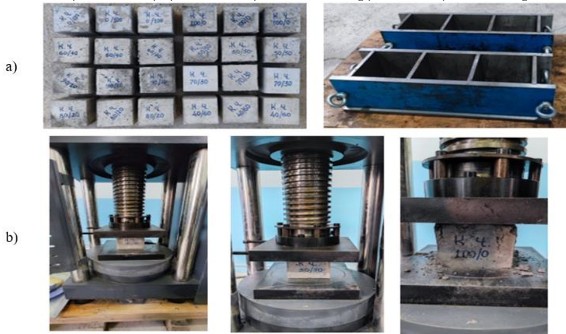
FIGURE 2. The prepared cube samples and their testing processes. Here: a – molds and cube samples prepared for testing processes; b – compression testing process of cube specimens.
