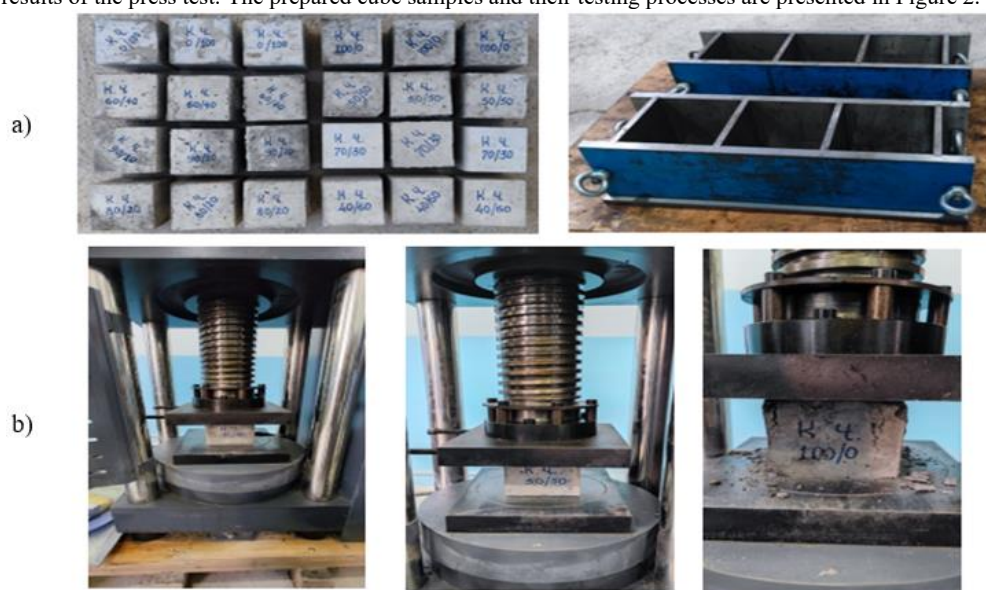
FIGURE 2. The prepared cube samples and their testing processes. Here: a – molds and cube samples prepared for testing processes; b – compression testing process of cube specimens.
