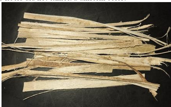
FIGURE 4. Fiber retted in sodium chloride (NaCl) solution.
