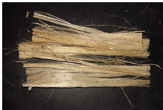
FIGURE 5. Alkaline solution of K_2CO_3 (potash) fiber steeped in water.
