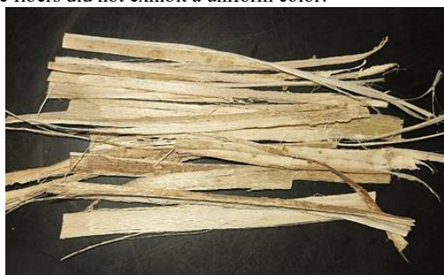
FIGURE 4. Fiber retted in sodium chloride (NaCl) solution.
