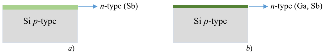
FIGURE 1. Principal schematic view of the samples after doping Ga and Sb impurity atoms into Si (a) Group I sample; (b) Group II sample.
