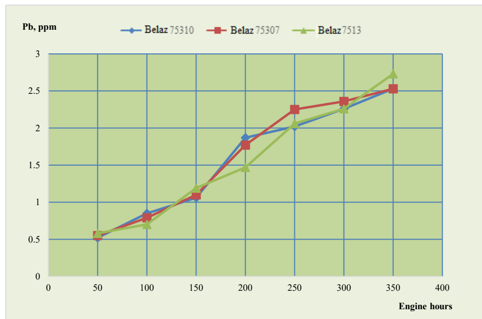
FIGURE 4. Dependence of lead (Pb) concentration in used motor oil—API CI-4, SAE 15W-40—on the operating time of dump trucks (engine hours).
