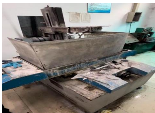
FIGURE 3. Electroerosion machine for sample preparation
