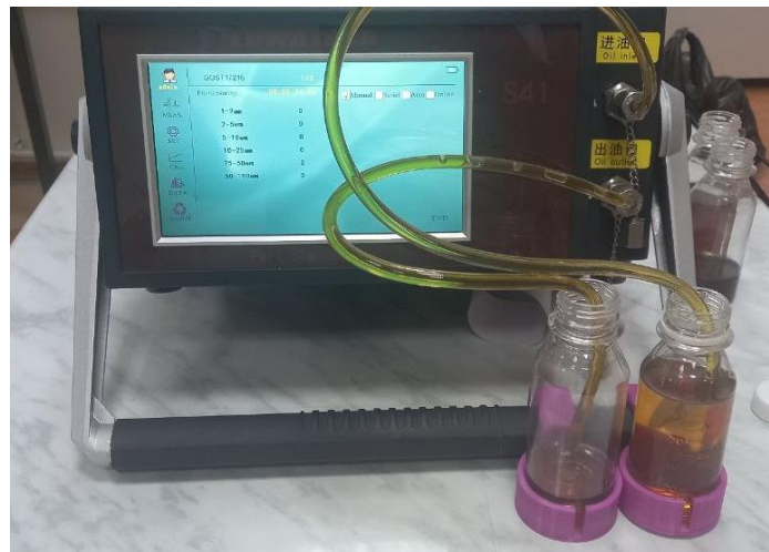
FIGURE 4. Process of analyzing working fluid on a Luwatech S41 mobile laboratory device for detecting contaminated particles
