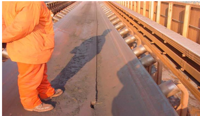
FIGURE 2. Longitudinal Tear in Conveyor Belts
