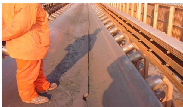
FIGURE 2. Longitudinal Tear in Conveyor Belts
