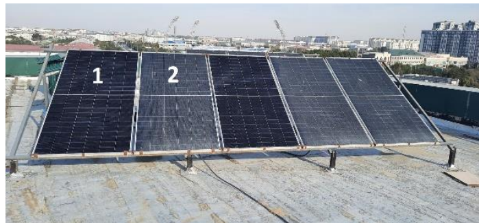
FIGURE 2. Procedure for measuring PV module parameters under real-world conditions 1– Photovoltaic module cleaned of dust, 2– Dust-soiled photovoltaic module
