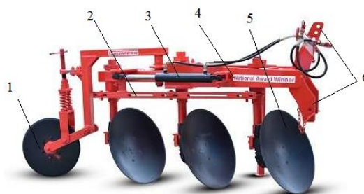
1 – support disc; 2 – drawbars; 3 – hydraulic cylinder; 4 – frame; 5 – disc working body; 6 – hitch mechanism.
