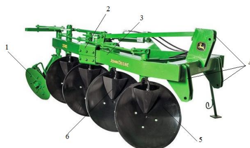
1 – support disc; 2 – drawbars; 3 – frame; 4 – hitch mechanism; 5 – disc working body; 6 – scraper.
