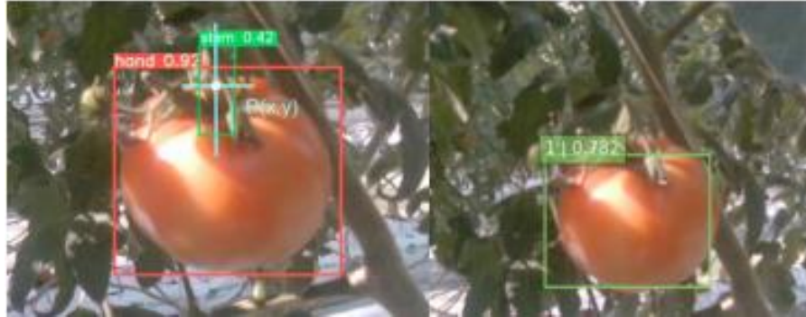
FIGURE 6. YOLO v5 (left) and SSD (right) quickly recognizes tomatoes and peduncles.
