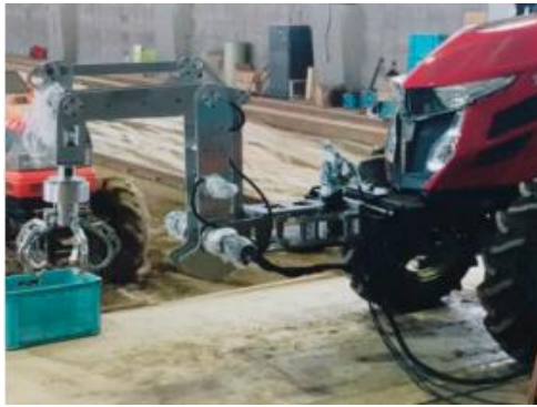
FIGURE 4. The robotic arm and end-effector
