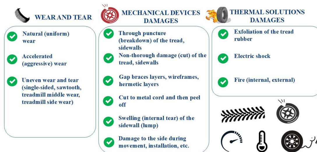
FIGURE 3. Improved classification of failure causes of large-size tires in quarry operation
