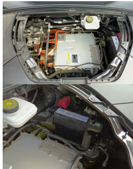
FIGURE 6. Physical layout of the BYD Song Plus power and control components
