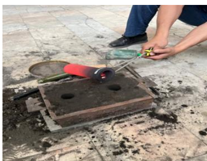
FIGURE 2. The process of pouring samples into sand-clay molds.
