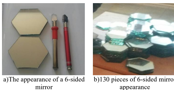
Figure 3. 6-sided mirrors with sides of 60 mm
