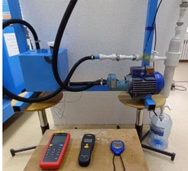
FIGURE 2. Hydraulic working fluid filtration stand
