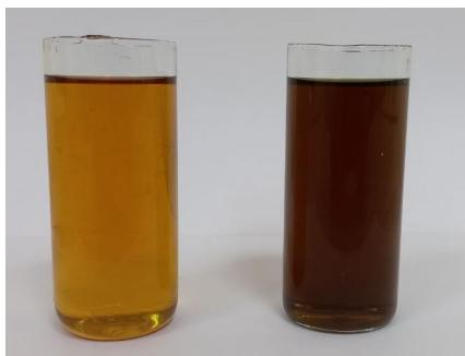
a - Hydraulic working fluid passed through the developed porous filter; b - Hydraulic working fluid passed through the hydraulic filter used in the excavator
