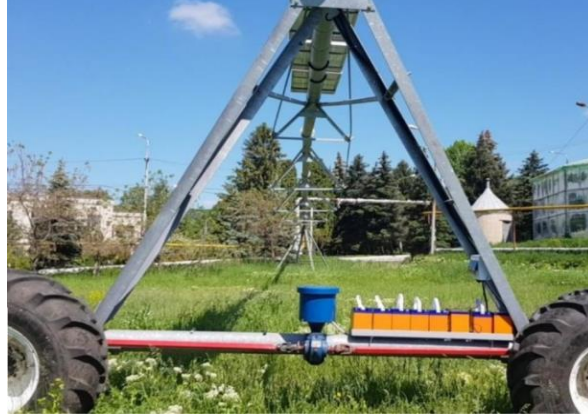
Figure 5. General view of the tested full-scale section of the irrigation machine equipped with photovoltaic modules and battery storage: 1 – SilaSolar photovoltaic modules with a total rated power of 600 W; 2 – Delta GEL battery units (12-55) with a total nominal capacity of 110 Ah; 3 – switched reluctance electric motor (gear motor) with a rated power of 500 W.
