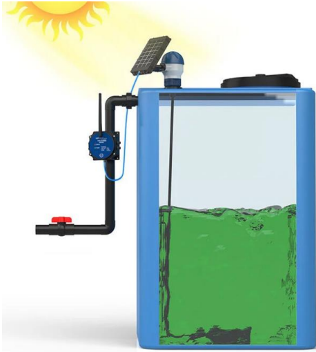
FIGURE 3. System for measuring the liquid level in an oil storage tank based on solar panels
