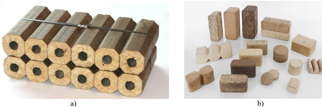
Fig3. The appearance of fuel briquettes made from waste; a) briquettes made from waste from oilseed processing; b) from leaves and other waste
