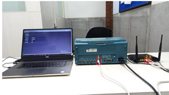
FIGURE 4. CONNECTION AFG TO A WIRELESS AREA NETWORK (WAN) VIA WIFI
