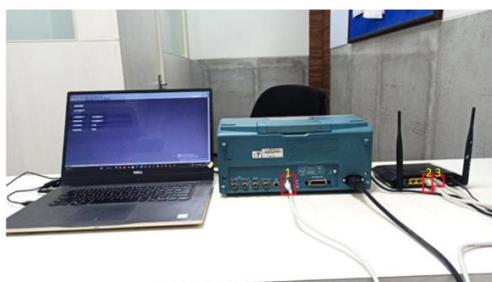
FIGURE 4. CONNECTION AFG TO A WIRELESS AREA NETWORK (WAN) VIA WIFI
