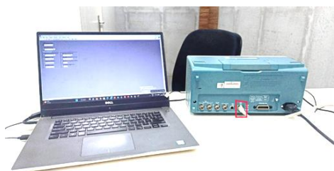
FIGURE 3 (A). CONNECTION AFG TO A LOCAL AREA NETWORK (LAN) VIA ETHERNET
