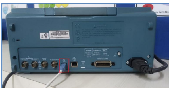
FIGURE 2 (A). USB INTERFACE OF THE AFG
