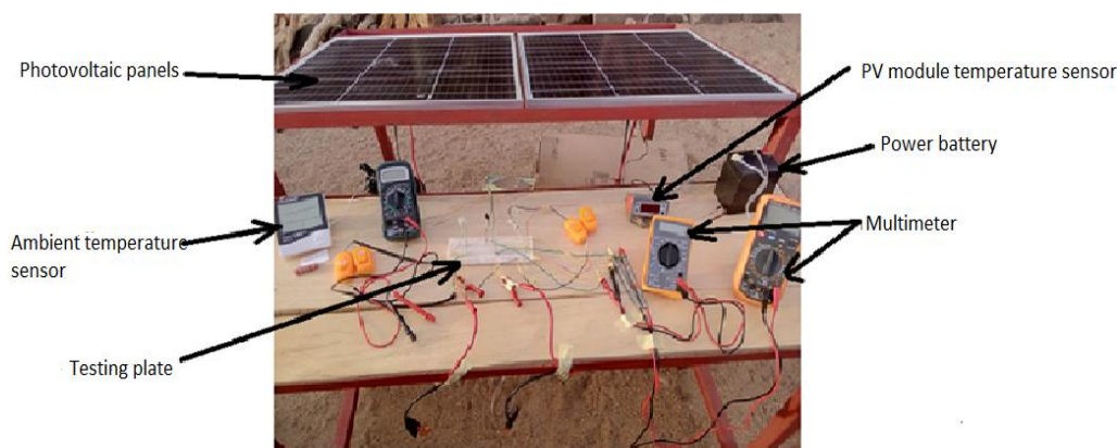
FIGURE 1. Experimental setup for the evaluation of the photovoltaic (PV) panel performance.
