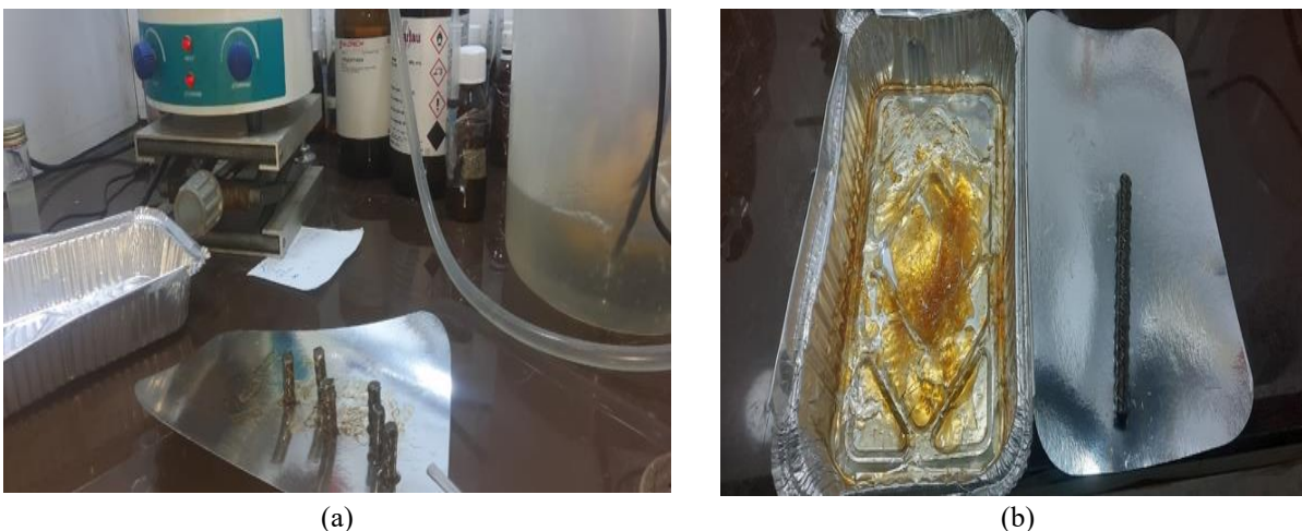
FIGURE 1. Photographic images of several steel rebars coated with hybrid monomers (a) steel rebars size 10 mm diameter \times 3 cm length, (b) steel rebar size 10 mm diameter \times 10 cm length
