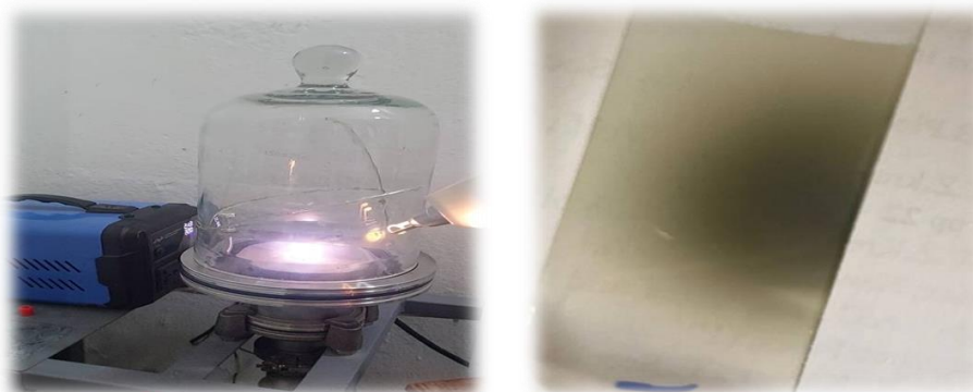
FIGURE 1. Photographic illustration of the prepared samples along with the pulsed laser deposition (PLD) system
